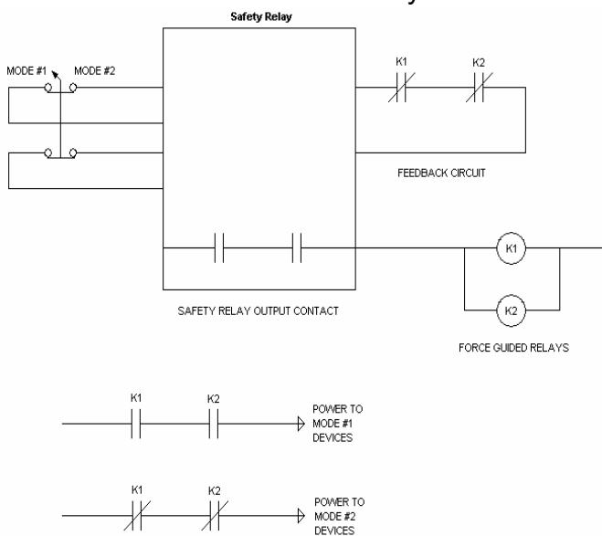
To determine if a relay is force guided, refer to the manufacturer's manual. Be careful with contact adder blocks, because some force guided relays don't have force guided adder blocks (Allen Bradley MB330, for example).
