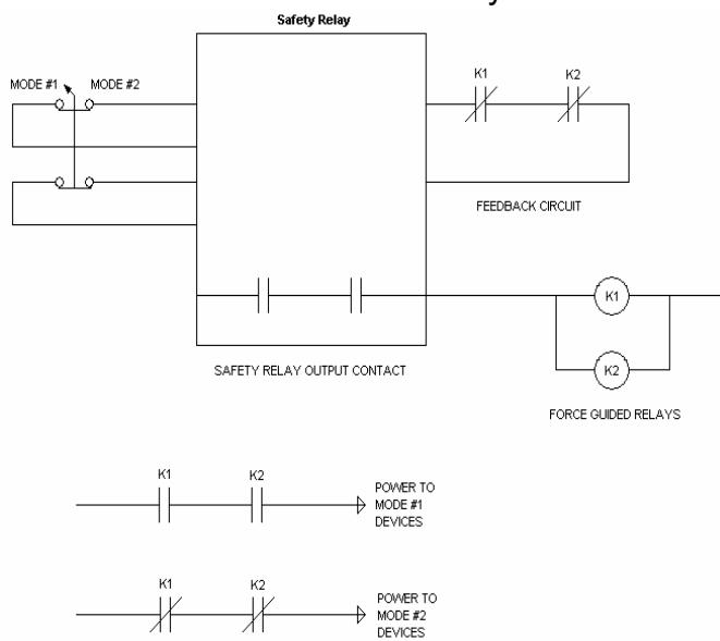
First, they are being used to expand the output contacts of the safety relay (similar to the safety expansion relay shown above). Note that two force guided relays are required in order to maintain control reliability. Secondly, the force guided relays are being used to interlock two modes of operation. This functionality could not be obtained using safety expansion relays, as they typically do not have reliable normally-closed contacts.
