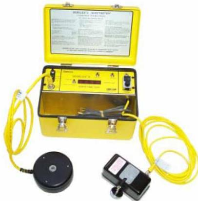
Wintek performs at least ten of these tests to obtain an accurate stop time. The data is used to calculate the safe distance of light curtains. The measurement process is quick, and allows us to physically measure the stop time of your machine rather than estimating it using combined delay times of all of relays and valves in your system. ⚡
